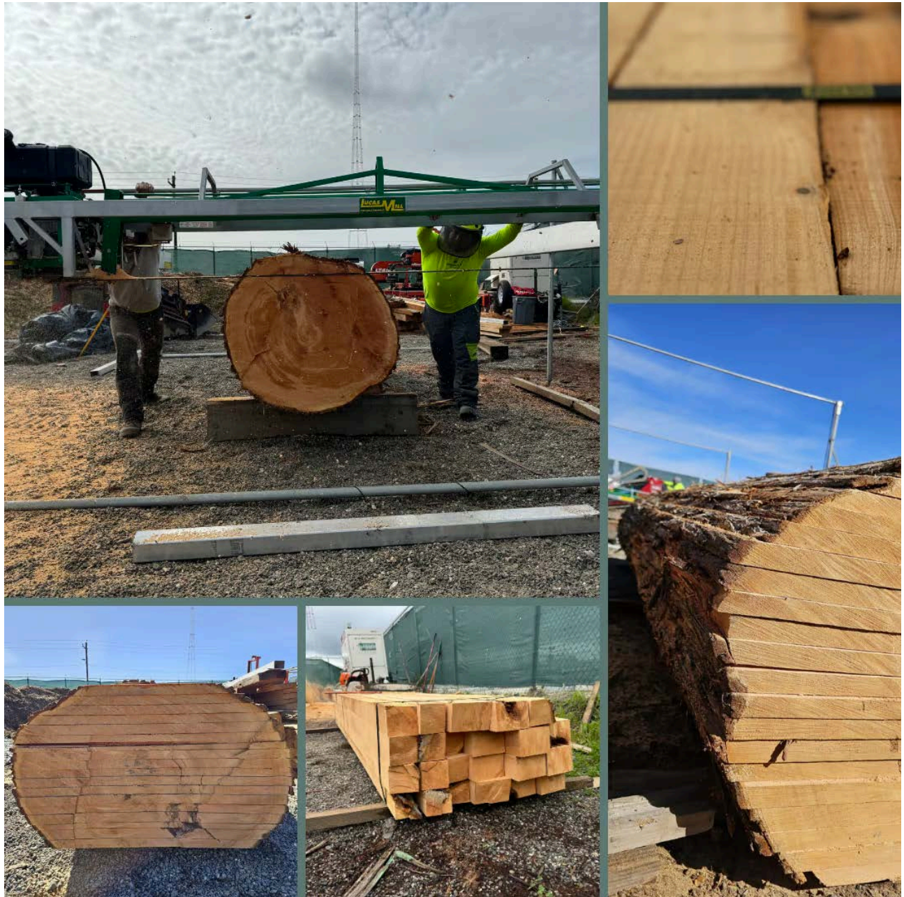
Milling Cypress on the Lucas Mill for Cypress Lawn Memorial Park
